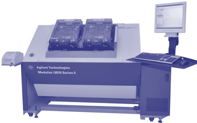
Figure 7.16: Example of a production test station.
